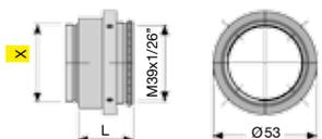
**ZR Extension rings L-Mount (M39x1/26" Leica)**
