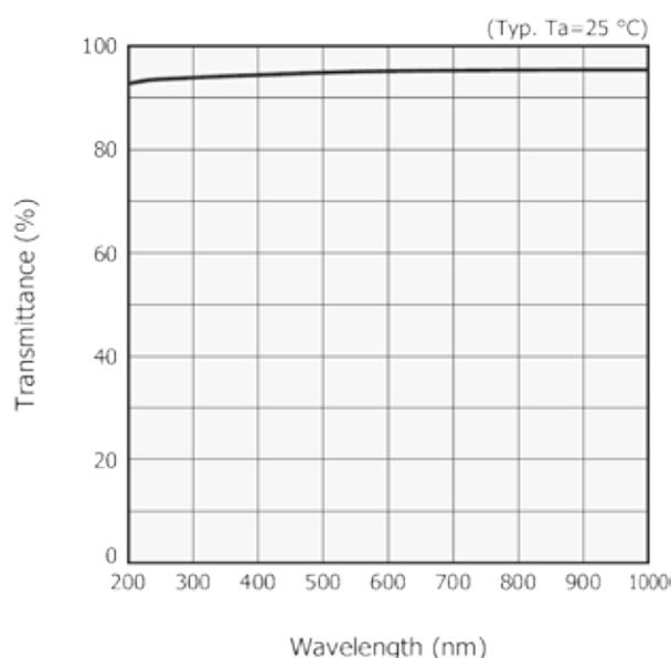
\* Spectral response will degrade depending on the transmittance of the quartz glass.
