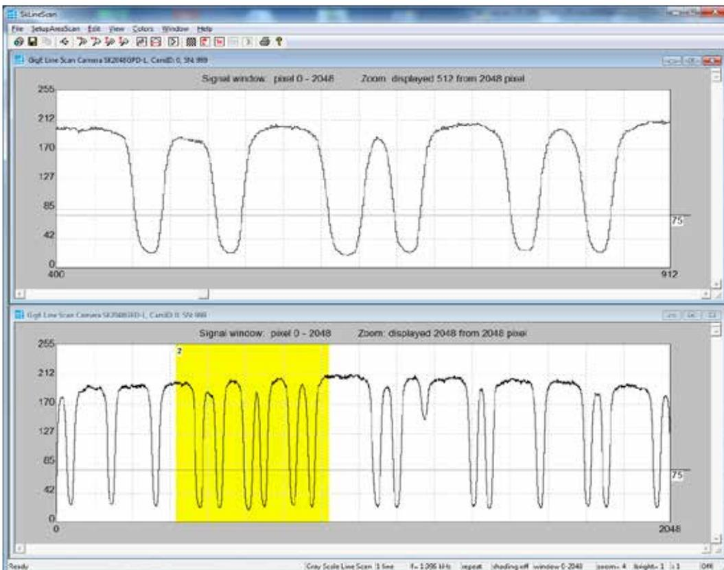
Line scan in split signal window: The upper frame shows an enlarged section of the lower frame.
