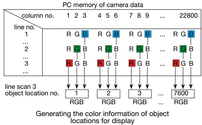
Triple line sensors require a precise synchronous translation of the object for the correct allocation of pixels. Also, the transport direction has to conform to the sequence of the line acquisition: first blue (B) then green (G) and red (R).
