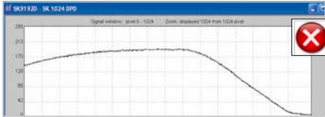
Sensor and optics rotated in apposition
