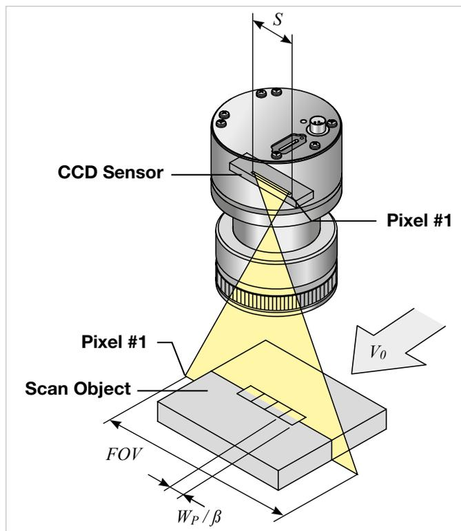
The optimum object scan velocity is calculated from:
