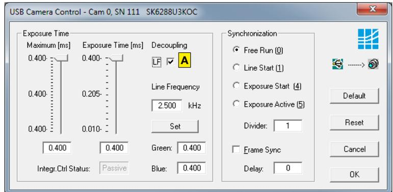
3. Reduce the integration times for the two color channels with the higher signals in order to align the Red, Green and Blue channels to the same level.
